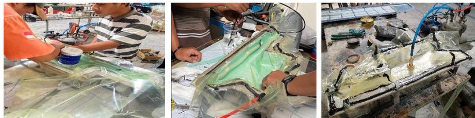
**Gambar 10. Pemasangan *vacuum bag* dipasang diatas serat Karbon Fiber glass**
