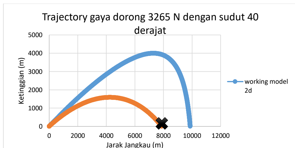
Gambar 8. Grafik trajectory perbandingan software Working model 2D dan Matlab Simulink
