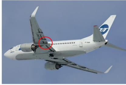
Gambar 1. Posisi crack wing Boeing 737-500 WL
