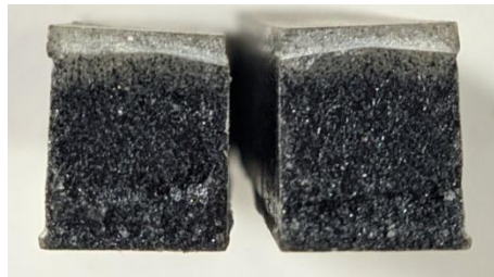
Figure 4. The results fracture of composite mixed matrix 50% epoxy and 50% iron sand Impact Test Results of 50% Epoxy Matrix Composite, 20% Horizontal Bamboo Fiber And 30% Iron Sand
