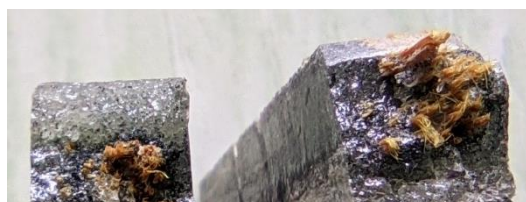
Figure 5. The results fracture of the composite matrix of 50% epoxy, 20% horizontal bamboo fiber and 30% iron sand
