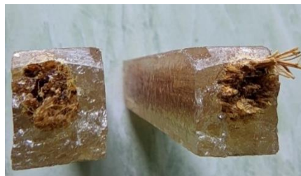
Figure 3. The results fracture of composite mixed matrix 50% epoxy and 50% horizontal bamboo fiber
