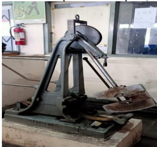
Gambar 5. Alat uji impact charpy
