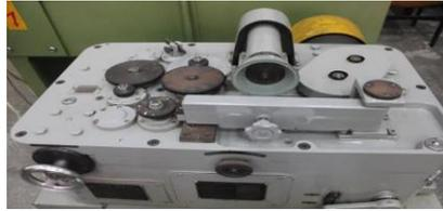
**Gambar 6. Ogoshi High Speed Universal Wear Testing Machine (Tyoe UAT-U)**
