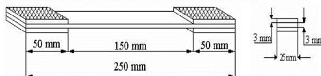
**Figure 2. Dimensions of ASTM D-3039**
