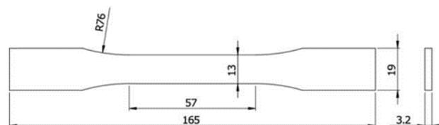
**Figure 1. Dimensions of ASTM D-638**
