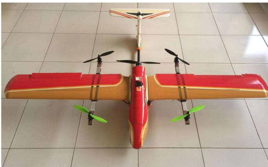
**Gambar 1.** Pesawat VTOL *Fixed Wing* Skywalker
