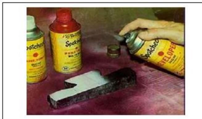
Gambar 13. *Penetrant Test*
