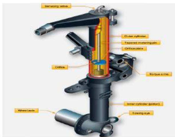
Gambar 4 Shock Strut (Sumber : www.airplane-picture.net )
