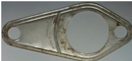
Gambar 1. Komponen Fuel Nozzle Gasket Pesawat Cessna Grand Caravan 208B
