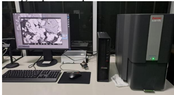
Gambar 6. Alat uji Scanning Electron Microscopy dan Energy Dispersive Spectroscopy
