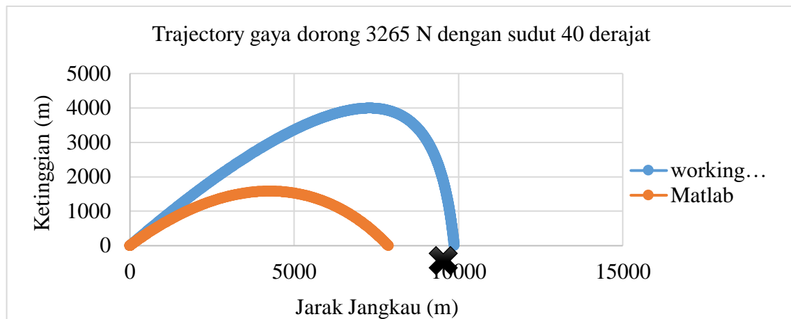
Gambar 12. Grafik trajectory perbandingan software Working model 2D dan Matlab Simulink
