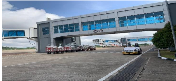
Gambar 1. Baggage towing tractor dan baggage cart terparkir di service road
